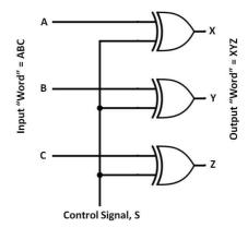
When the control signal is 0, then the output word XYZ is the same as the input word. However, when the control signal is 1, then the output word is A'B'C', with the bits inverted.
