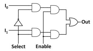
The outputs from the existing AND gates now enter two additional AND gates. If the Enable input is 0, neither  $I_0$  nor  $I_1$  get through. If the Enable input is 1, then the selected input gets through to the OR gate.
