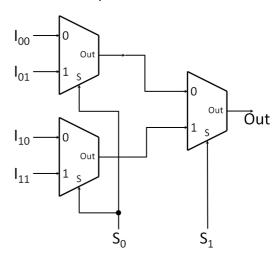
Some thought about how MUXs work, reveals the following truth table. This table shows which line is output for a given combination of enable inputs.
