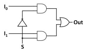
We see that the circuit consists of two AND gates, one OR gate, and one NOT gate. The gate symbols are as follows:
