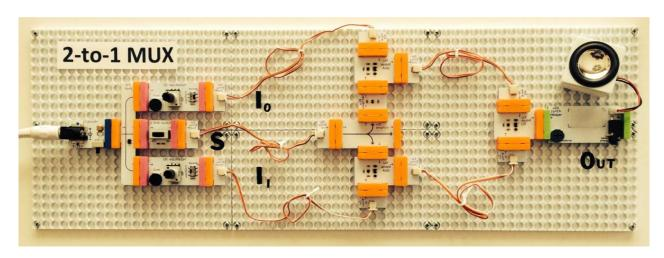
**ACTIVITY 1:** Construct a 2-to-1 MUX without Enable
