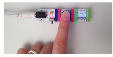
An activated input can be described in many ways. When we press a button before a motor module, the motor shaft will turn. In this example, energy passes through the input and can now flow on to the next module.
