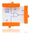
The NOR module is a logic gate with two inputs and one output. NOR stands for NOT OR, meaning the output of the OR module is inverted. With the NOR module, the output is on when both inputs are off, or false. If either or both inputs are on, the output will be off, or false. The NOR gate is good for projects in which you want the output to be on unless one or both of its inputs are triggered.
