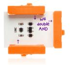
The AND module is a logic gate with two inputs and one output. In order for the AND gate to output an on signal, both inputs need to be on at the same time. When this happens, you are able to activate any output module like an LED, a DC motor, or a buzzer. The AND module is a good option for projects in which you want two actions to trigger another.
