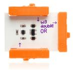
The OR module is a logic gate with two inputs and one output. In order for the OR gate to output an on signal, the first input, the second input, or both inputs need to be on. When both inputs are off (inactive), the output is off. The OR is good option for projects where you want to detect two inputs but don't care which input is activated.
