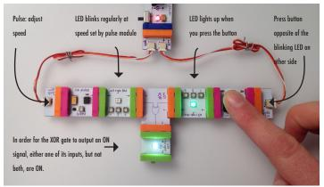
Set the pulse to whatever speed you like. The LED that follows the pulse will now blink at a regular rate. Press the button (your second input) in between the beat of the pulse. You will know that you are keeping the upbeat when your output light remains on and does not blink out. If you change the speed of the pulse, you change the rate of the metronome. See how fast or slow you can go to keep a syncopated rhythm.
