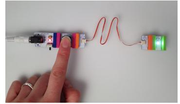
WIRES CARRY SIGNAL FROM ONE MODULE TO THE NEXT
