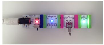
WIRED IN SERIES WITH THE SWITCH ON. THE LED BIT IS ON.
