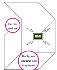
$\textbf{Circuit: power + split} < \substack{ \text{roller switch + wire} \\ \text{light trigger + wire} } > \texttt{NAND + buzzer}$
