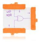
The XOR module is a logic gate with two inputs and one output. In order for the XOR gate to output an on signal, either one of its inputs, but not both, are on. The XOR is called the exclusive OR because it is similar to the OR gate, but only outputs a signal when one input is on at a time. The XOR is great for projects in which the activation requires input alternation.
