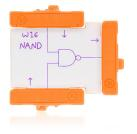
The NAND module is a logic gate with two inputs and one output. NAND is short for NOT AND which is the combination of an AND gate where the output is inverted. The NAND only outputs an off signal when both of the inputs are on, or true. If both inputs are off, the output signal will be on.
